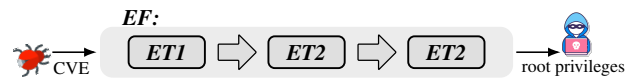
Figure 1: The exploitation flow EF is a vulnerability-agnostic chain of exploitation techniques ET , with one ET elevating a primitive to a more powerful form [8]. EF leverages the capabilities of a vulnerability to gain root privileges ultimately.
