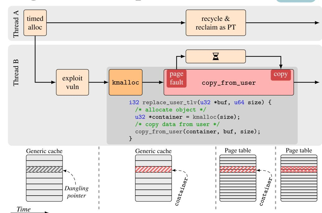
SLUBStick exploits a heap vulnerability for a page-table manipulation, by first creating a *dangling pointer*. It then reclaims the pointer's memory for container, where writing via copy\_from\_user causes a slow page fault. SLUBStick recycles the cache's page and reclaims it as a page table, where copying then overwrites page-table entries.
