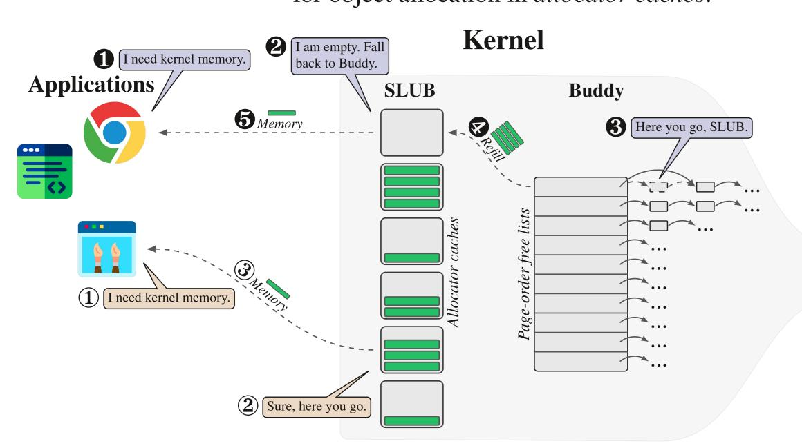
**Object Allocation.** Applications use the SLUB allocator caches: - Fast path: on a memory allocation (1), the allocator cache has free
