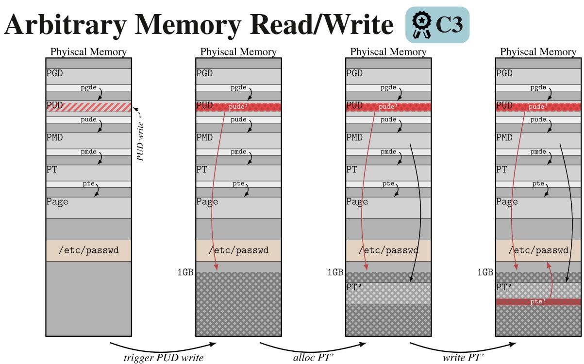
SLUBStick converts a single-shot page-table manipulation to an arbitrary **physical read/write**: It *triggers the PUD write* so that the user address with pude' refers to the first physical GB. It then *allocates PT'* and *overwrites* a PT' entry with pte'. The user address with pte' now refers to an arbitrary physical location, allowing the arbitrary physical read/write.
