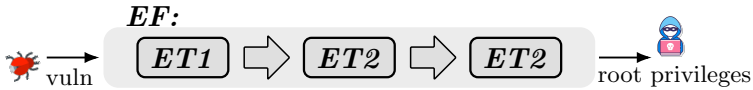
Figure 2.3: The exploitation flow EF is a vulnerability-agnostic chain of exploitation techniques ET . Each ET is a reusable and reasonably generic strategy to turn one exploitation primitive to a more powerful one [15]. Ultimately, the EF leverages the capabilities of one or more vulnerabilities—such as UAF write—to gain root privileges—such as via an arbitrary read/write primitive.
